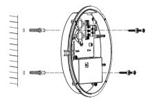
Fix the back housing on the wall or ceiling using the screws.
