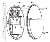
Connect the DC plug (if with emergency, connect the plugs between the battery and driver) put back the cover to the base plate and fix it with the screws
