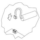
Connect battery to converter
