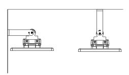
Check that the fixing is correct before connecting the wiring. If the luminaire is held securely, proceed with the connection of the luminaire to the power supply.
