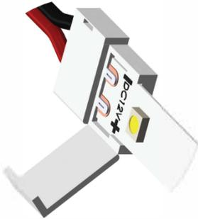
Connect LED tape to the power by sliding in and ensuring that it locates under the two metal tabs. The RED wire must align with the + on the LED tape.
